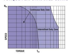
**NOTE:** Continuous torque specifications obtained with motor mounted to an 8.5"x12"x 0.25" aluminum plate at 25°C ambient. Typical values are within  $\pm 10\%$  of rating.
